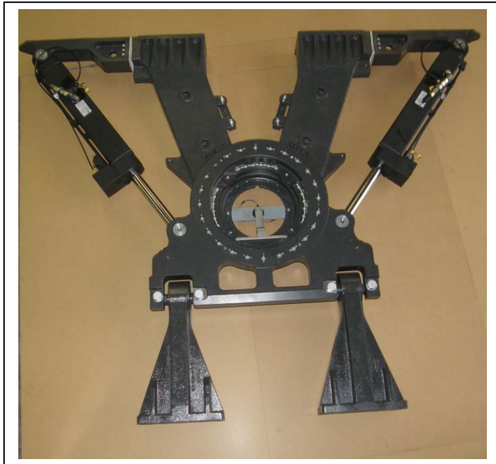
Fig.5 ARTIC-O-MAT II 350 IC equipped with Integrated cylinders.
